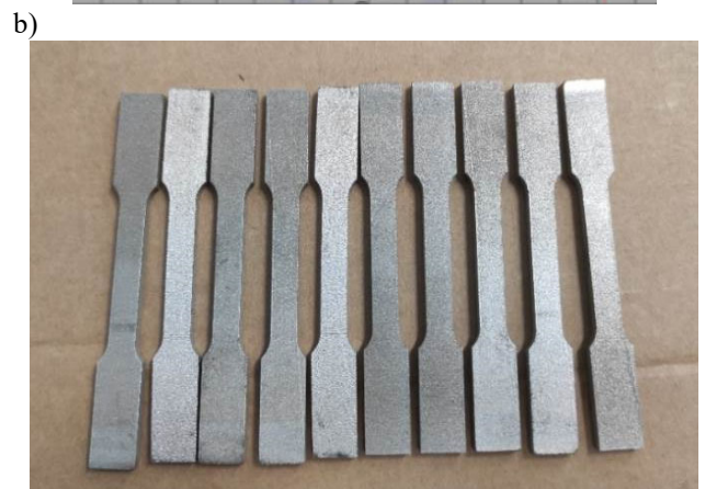
Fig. 3. a) Visualisation of the arrangement of samples for static tensile testing during printing; b) Samples after 3D printing with DMLS technology prepared for static tensile testing
